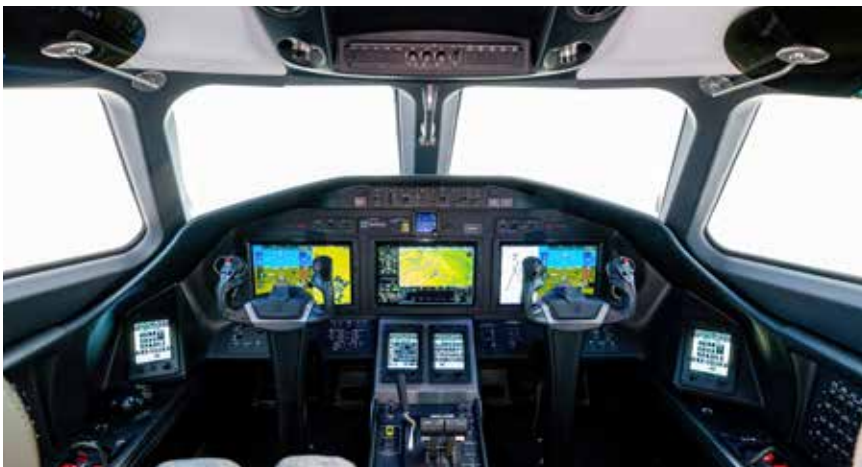
The Longitude's flight deck features Garmin's G5000 avionics suite with four touchscreen controllers.
