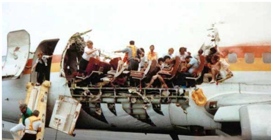
Figure 1. The 1988 Aloha Airlines Incident Occurred due to Lap-Joint of Fuselage Fatigue Failure
