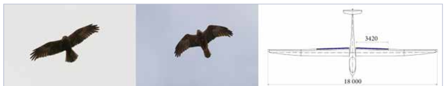
Figure-5. Long-Legged Buzzard decreases wing area by 20% during gliding flight which optimizes gliding performance. This application can be seen in the LAK-17 Experimental Glider as mini flaps extend in the thermal.
